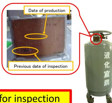
Filling of vessels overdue for inspection with LN<sub>2</sub> is prohibited
